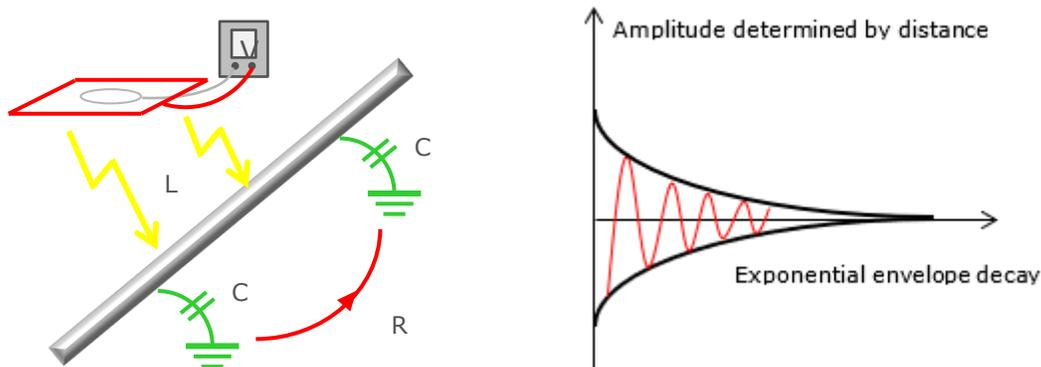
Figure A1- 2 Illustration showing the effects of capacitive coupling.
