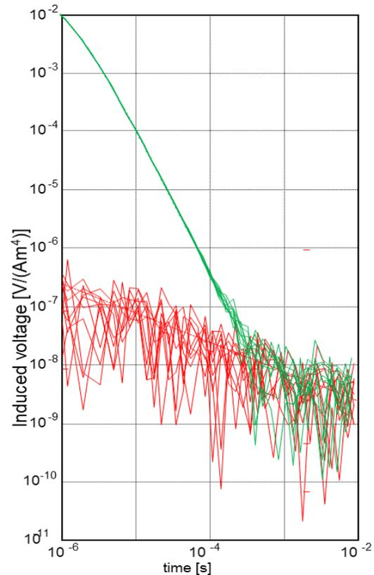
Figure A1- 3 An Example of decay curves created by a TEM system (Green curves) and the background noise floor (Red curves).
