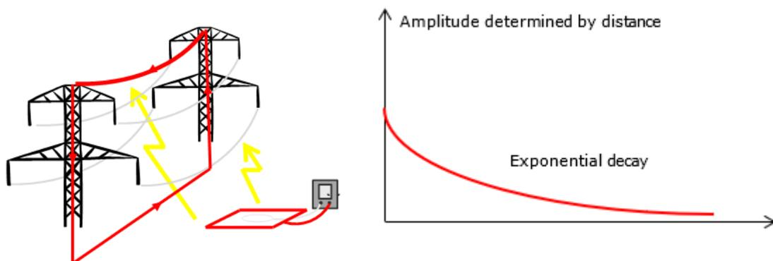
Figure A1- 1 Illustration showing the effects of galvanic coupling.
